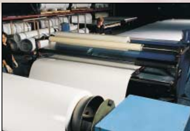
The nip roll press technique guarantees a permanent bond.
